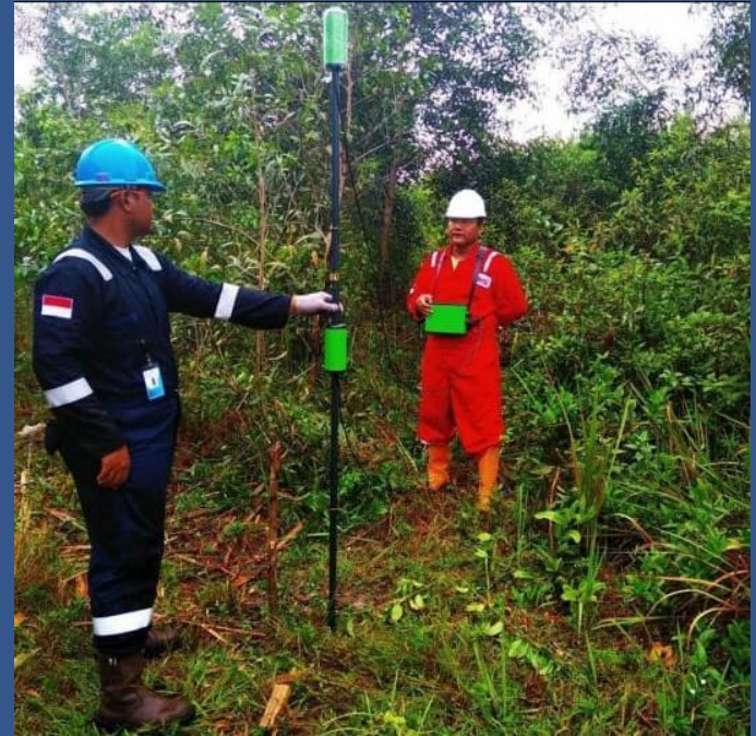
Geomagnetic method for pipeline tracking at Senipah for ENI, Kalimantan
